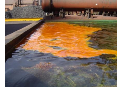
Wash oil spill
