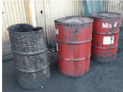
Drum damaged, no lid, full of waste oil & un- bunded
